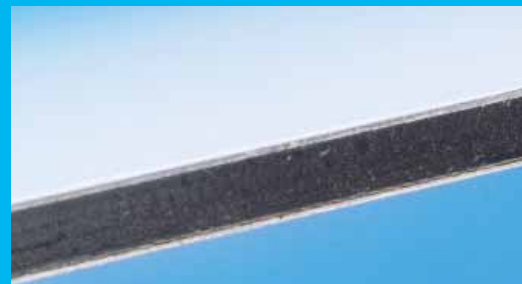
Aluminium Composite - a sandwich of 0.3mm aluminium with a 2.4mm polyethylene core
